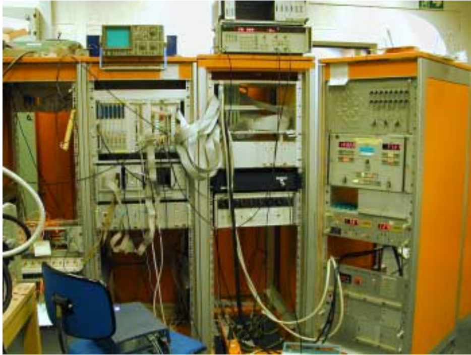
Figure 2 The new signal processing and control hardware for the Tromsø UHF radar.
