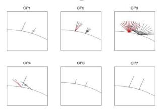
The circles denote the common volumes sampled by the mainland tri-static system. The mainland system is represented by the trace on the right and the ESR system by the trace on the left. In the case where the ESR 32m dish is not pointing field aligned a blue trace indicates the 42m antenna and a red indicates the 32m antenna. The table in section 3.1 of this guide indicates the default experiment type that will run with each CP.
