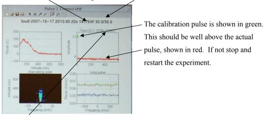
The system temperature is shown above the top right hand plot in the square brackets. If this number is 'NaN' or extremely high (ie. So the building would have to be on fire!) then this is an indication that what forever reason the system is not synchronised. YOU MUST THEREFORE STOP AND RESTART YOUR EXPERIMENT. This should hopefully fix the problem.
