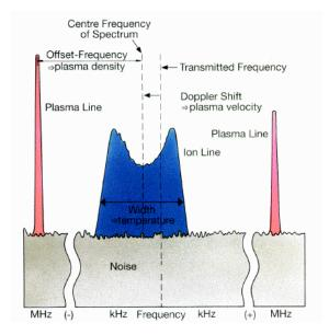
The total returned power depends on the number of electrons and gives an estimate of the ionospheric electron concentration, the width of the spectrum depends on the ratio of the ion temperature to the ion mass, and the overall shift of the spectrum corresponds to the bulk drift motion of the ions (the plasma velocity).
